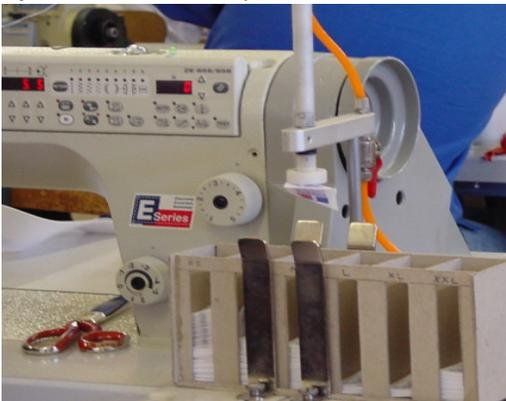
This is a Venturi Tube which uses air pressure to pick up the labels, so there is no fiddling around while picking up the labels.
